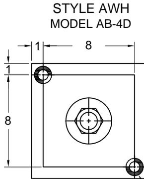
ELASTOMERIC GROMMET FOR 1/2 ANCHOR BOLTS (2 TYP)
